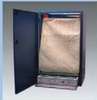
Option B: 36" Pocket Envelope Bag 4" 30% ASHRAE Filter 1" Metal Mesh
